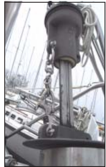
Figure 4 - Foil “car” attaches to genoa head
