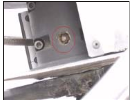
Figure 1 - Furler grease fitting
