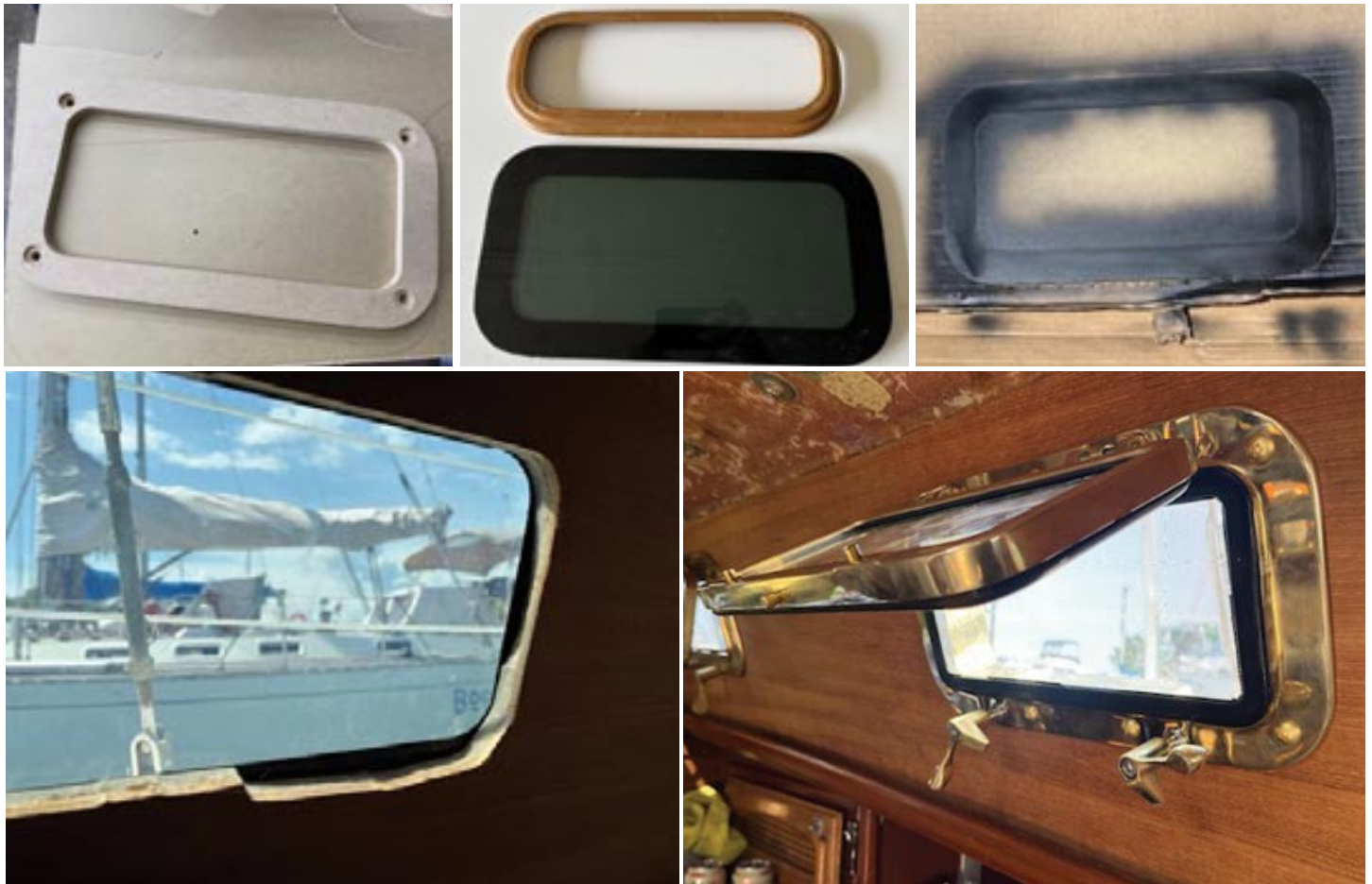
Port template, size difference, painting the border black and the slip up with the router brings new bronze ports to the salon
