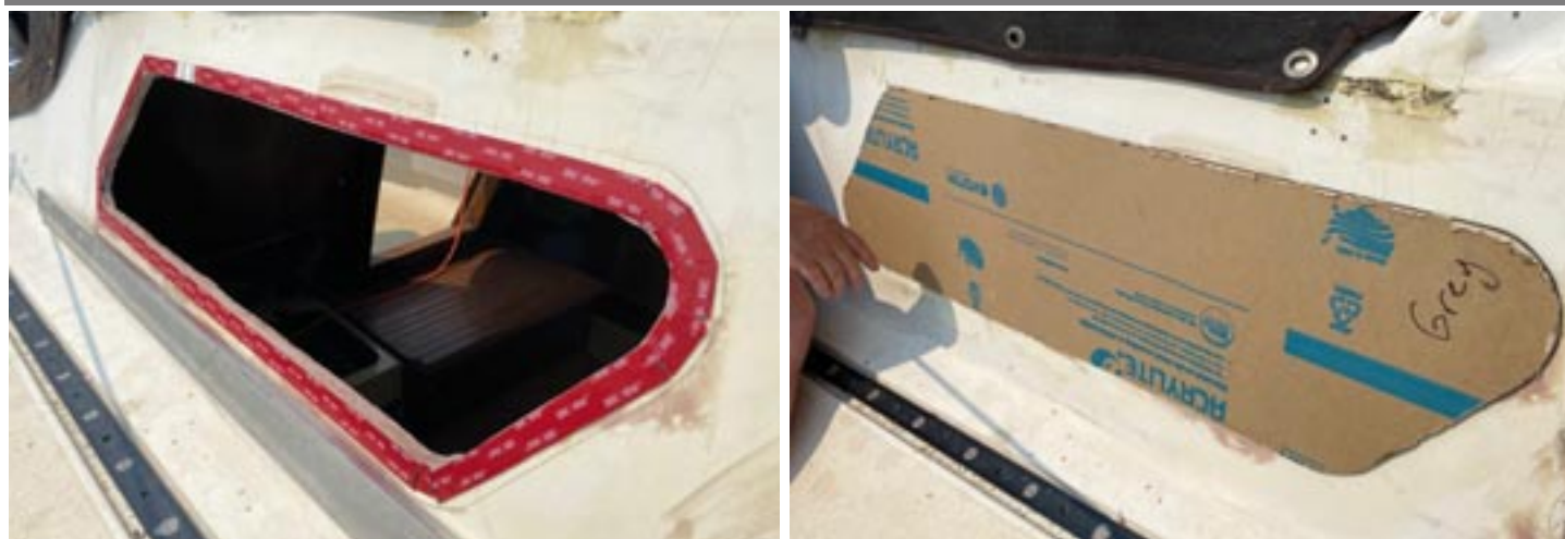
Ports with VHB tape and acrylic placed - ready for peeling
