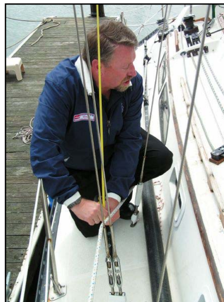
At the 2007 Sail Trim Clinic, guest speaker Michael Whitfield demonstrates how to check if the mast is centered in the boat and how to check mast rake.
