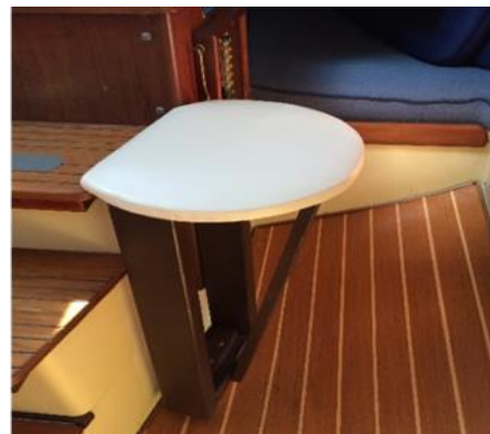
Next – tilt stool vertical and push down to seat the bolts into the floor block and attach eye
