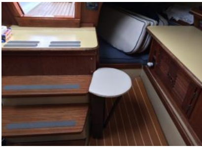
To install – tilt stool at an angle and align the two bolts with floor block.
