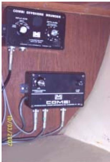
**Figure 1 - Combi Speed-Depth Measurement System**
