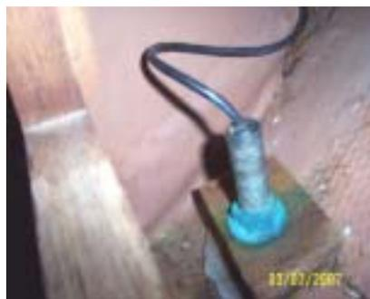
**Fig 4 - Old transducer interior**
