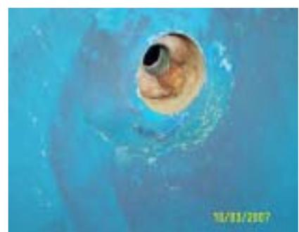
**Fig 5 - Old transducer thru-hull**
