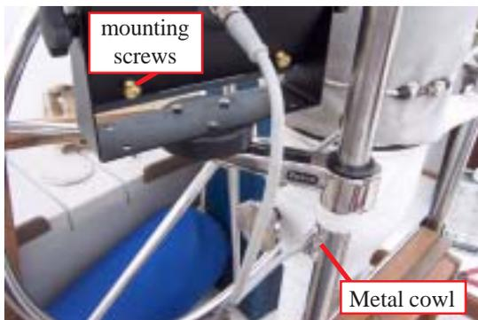
**Fig 13 - Display mounting screws & connector**
