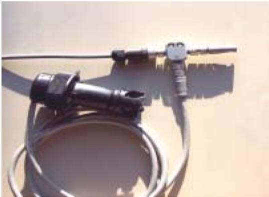
**Fig 10 - Transducer connected to bus via a terminated tee connector**
