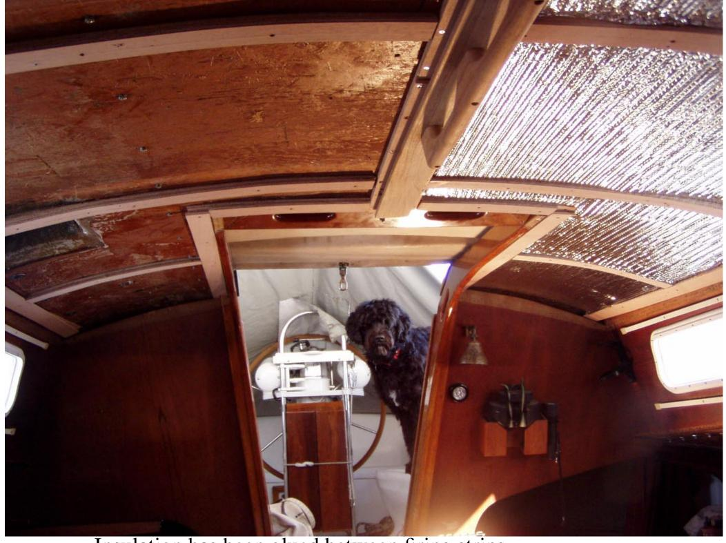
Insulation has been glued between firing strips
