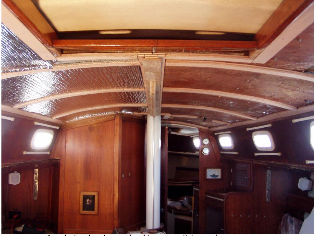
Insulation has been glued between firing strips
