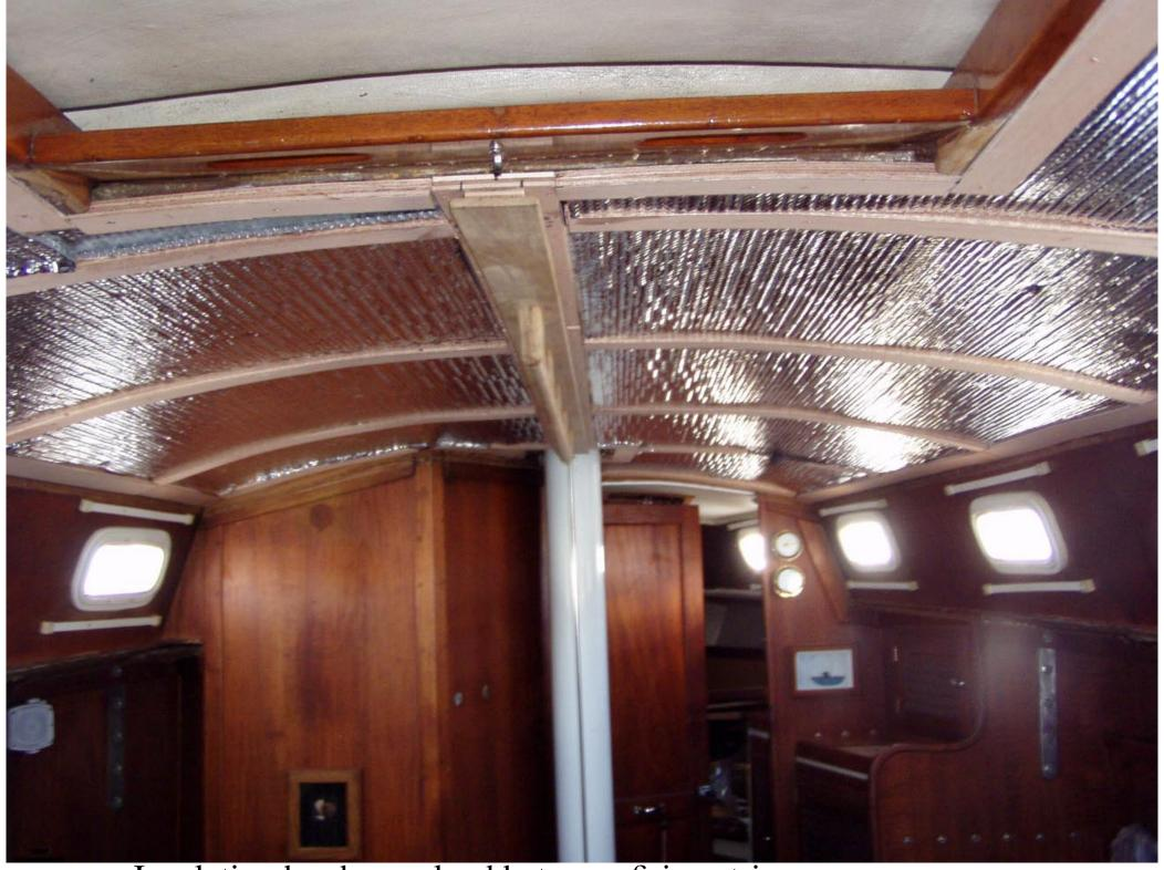
Insulation has been glued between firing strips
