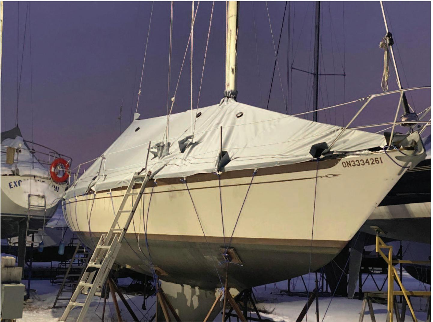
unstepped the mast, we'd be able to cover the boat more easily, but not without other issues: the hassle of stepping and unstepping the mast; the expense of tarps big enough to cover the boat as they tend to wear out quickly; building a framework to support the tarp so that snow would slide off.
