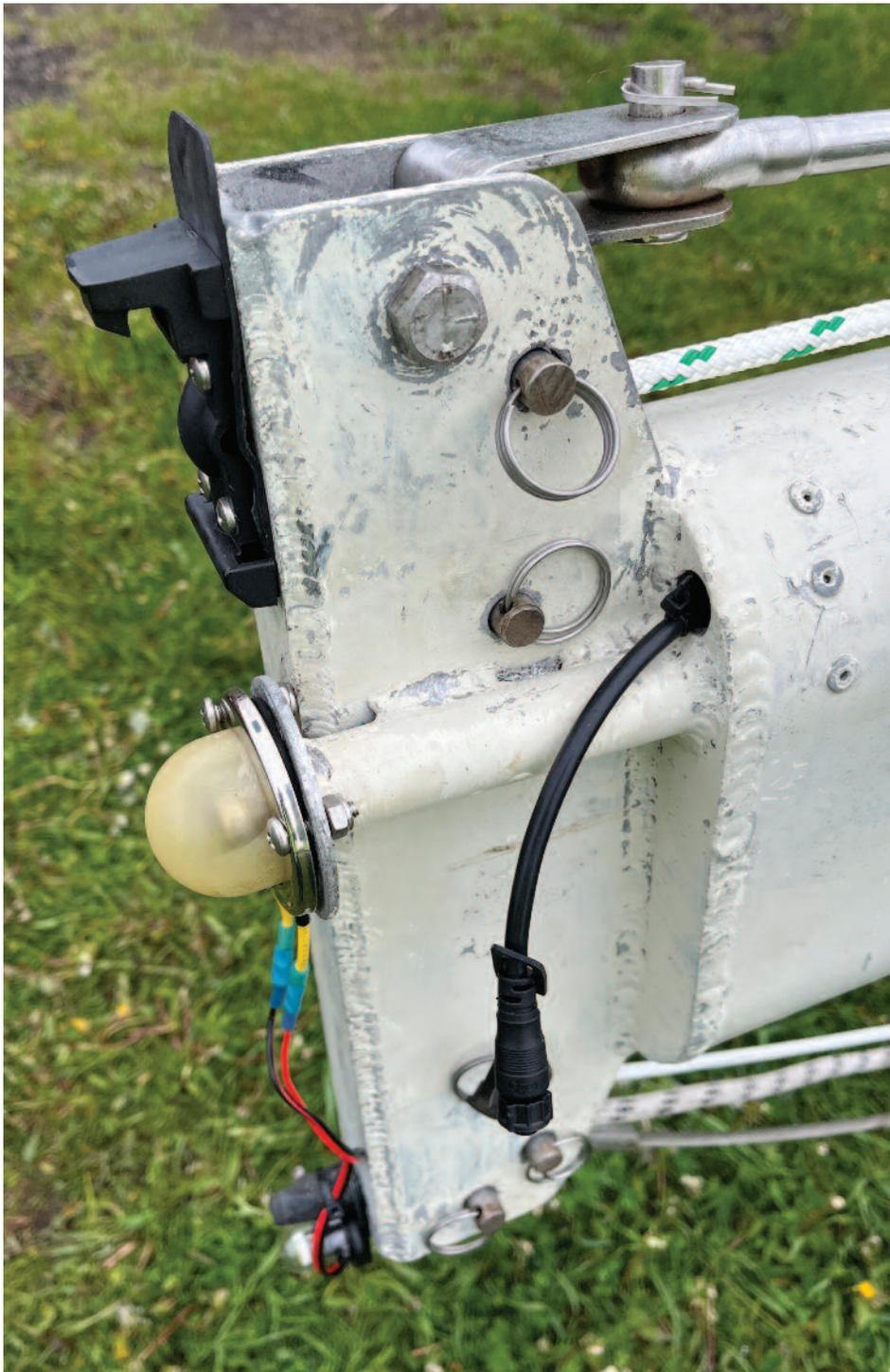
one with a wired wind sensor. While the wireless wind instrument probably would have worked just fine, going with wired ensured no hassles with batteries or signal reception.
